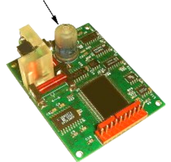
Typical digital compass module containing a Spectron Tilt Sensor for compensation
