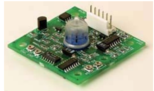
Figure 7. The Spectrotilt II dual-axis inclinometer uses a single dual-axis sensor (center). A matching-hole pattern for the sensor electrodes (pins) is incorporated into the circuit board. Soldering the sensor to the circuit board provides both the electrical and mechanical connection.
