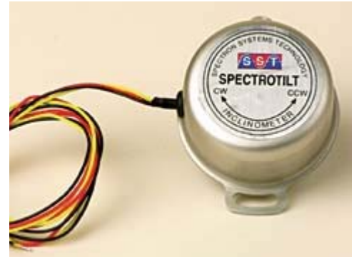
Figure 6. The Spectrotilt electronic inclinometer has a \pm 60^\circ total range, allowing use in widely varied applications. Onboard linearity and temperature error correction enable absolute measurement accuracies as high as \pm 0.3^\circ . The mounting features and package size are industry standard.
