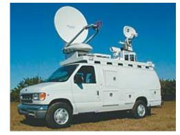
appropriate satellite and locked into place. For mobile apps such as satellite news gathering, alignment is trickier. And errors on the order of fractions of a degree can cause signal degradation, loss, or failure to acquire.
