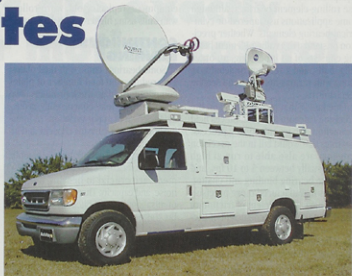
Mobile satellite applications such as news-gathering vans need accurate position feedback from tilt sensors to align the antenna with the appropriate satellite.
