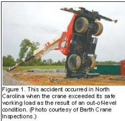
Figure 1. This accident occurred in North Carolina when the crane exceeded its safe working load as the result of an out-of-level condition. (Photo courtesy of Barth Crane Inspections.)
