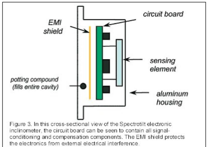
Figure 3. In this cross-sectional view of the Spectrotilt electronic inclinometer, the circuit board can be seen to contain all signal-conditioning and compensation components. The EMI shield protects the electronics from external electrical interference.
