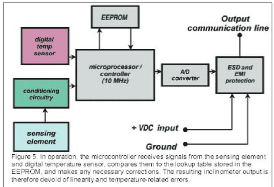
Figure 5. In operation, the microcontroller receives signals from the sensing element and digital temperature sensor, compares them to the lookup table stored in the EEPROM, and makes any necessary corrections. The resulting inclinometer output is therefore devoid of linearity and temperature-related errors.
