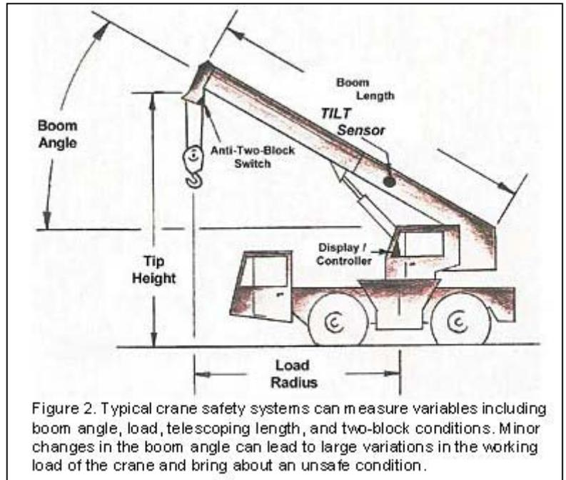
Figure 2. Typical crane safety systems can measure variables including boom angle, load, telescoping length, and two-block conditions. Minor changes in the boom angle can lead to large variations in the working load of the crane and bring about an unsafe condition.
