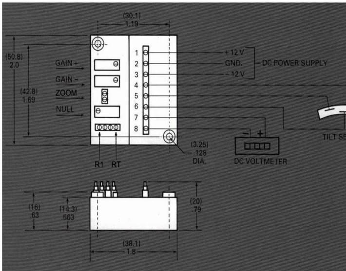
1. Connect the tilt sensor to the MUPI-23 on terminal numbers 1, 2, and 3 per diagram.
