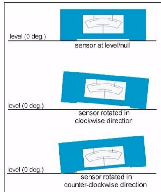
6. Turn 'Sensor Null Adjustment' potentiometer until output on Digital Voltmeter reads 0.000Vdc (see below for potentiometer locations).
